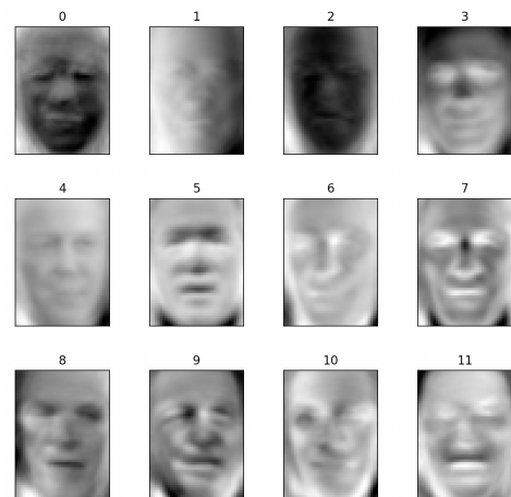
Figure 4: The first 12 eigenvalue components from the LFW image dataset
